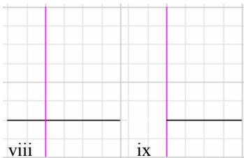
Undo. Trim Break is the most commonly used trimming tool. (viii) Trim Break and select one line to be the "break." (ix) Click the intersecting line on the side that is to stay.
